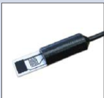
SHS - Special probe for condensation detection. Condensation sensor signals 1 when condensation causes wetting. Operation at 0...50°C Dimensions: 43mm x 10mm
